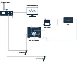
Illustration and setup principle to perform fluid recirculation with an Elveflow MUX Recirculation valve. The detailed protocol for this application can be found in the MUX Recirculation valveuser guide.
